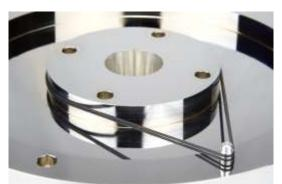
It is essential to have clean hands when handling the drive belts, and also recommended that you clean the platter drive hub and motor drive pulley before installing the belts. Using isopropyl alcohol cleaner is suitable for this purpose.
