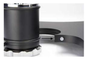
Insert the motor into the designated cut-out in the main chassis, ensuring that the lower rubber O-ring on the motor aligns with the groove on the side of the chassis.
