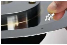
To install the drive belts, you must first attach them to the platter using the designated belt fitting pin.
