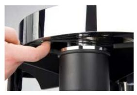
With a gentle touch, lift the platter edge to expose the motor pulley. Rotate the platter to engage the belts with the grooves of the drive pulley. Using your finger, hold the drive belts against the underside rim of the platter, and then remove the fitting pin. Finally, let go of the drive belts, and they will be secured in place.
