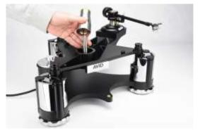
Now, as previously directed, reinstall the main bearing, ensuring that you are extra careful not to harm the sapphire bearing by dropping it too hard onto the bearing ball.
